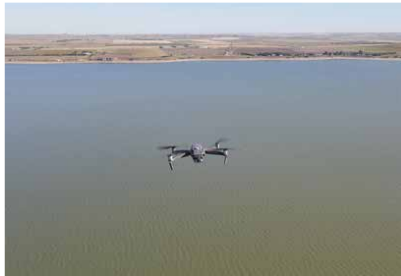
One of CCI's drones used for drilling fluid release monitoring of the watercourse
