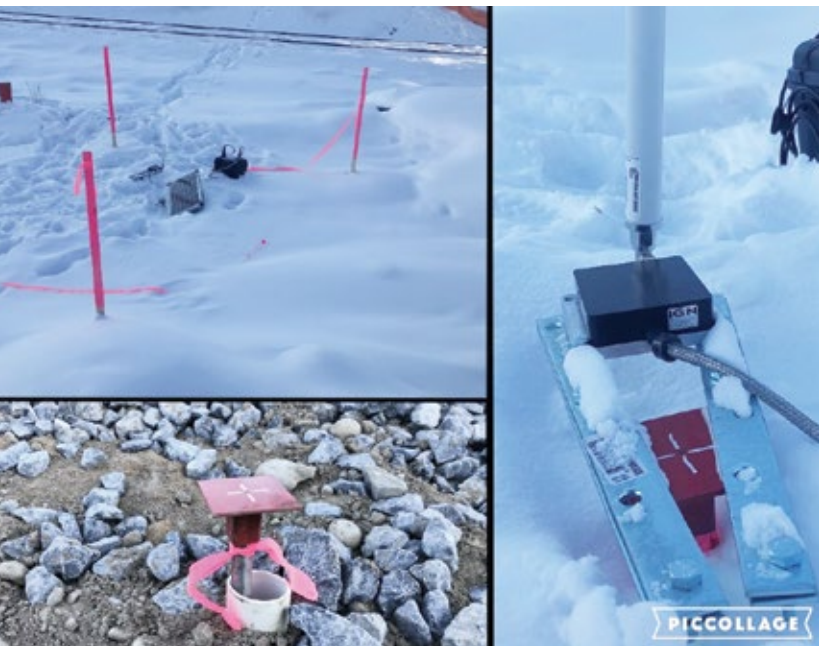
Figure 2: Robust self-contained GPS units that can be utilized to monitor settlement remotely
